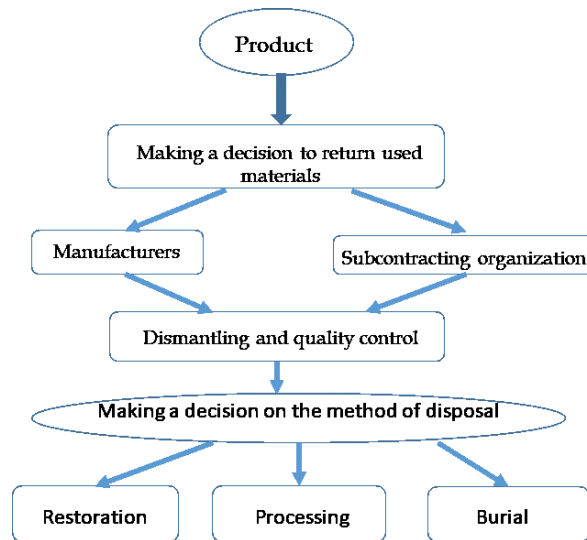
Fig. 1. Model of decision-making regarding the choice of the method of product disposal at the end of its use, taking into account environmental and economic factors.
